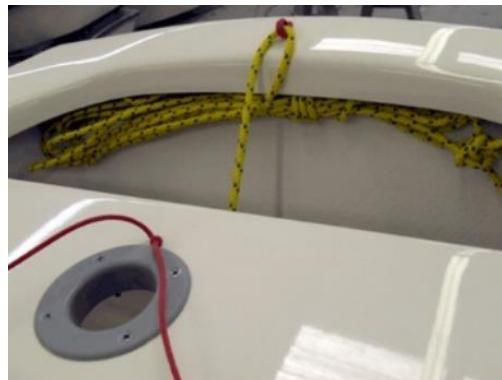
When boats are towed, they usually do this in a daisy chain configuration, so you also want to make sure there is a bowline (loop) on the end of the line and it's coiled up and stuffed under the rail. (right photo above).
